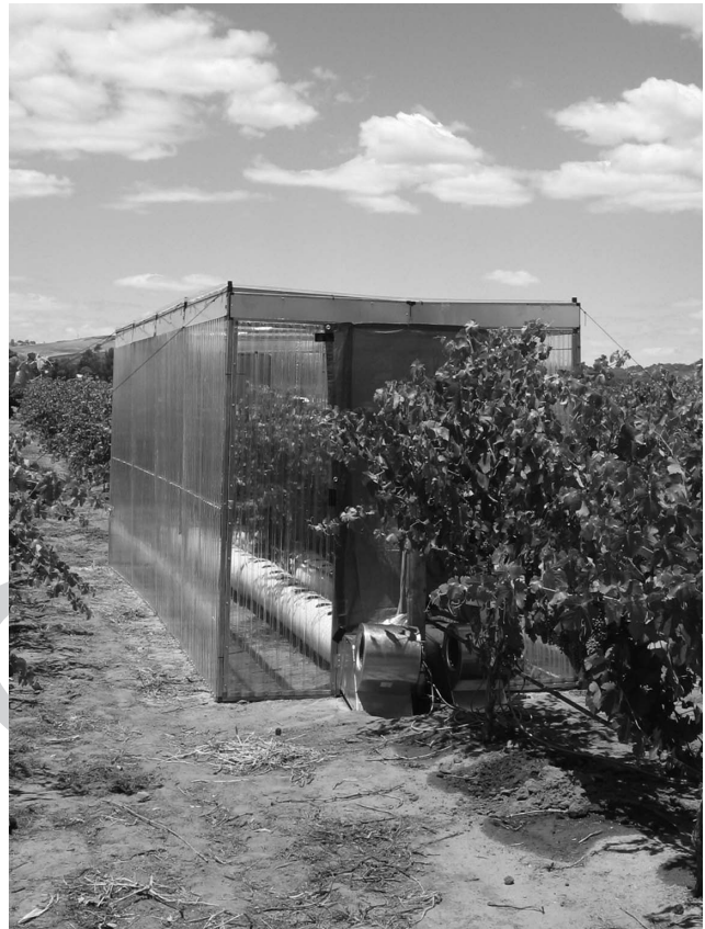
Fig. 1. Heat chamber combining passive heating (greenhouse effect) and active cooling (fans) to control daytime temperature.
